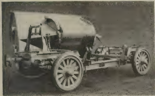
A THREE-TON DROP-FRAME TRAILER.
